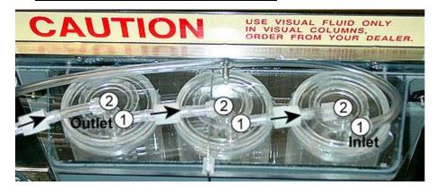
Step 3: Re-Affix sleeves onto Visual Barbs, tightening hand tight. Use arrows as flow guide.
